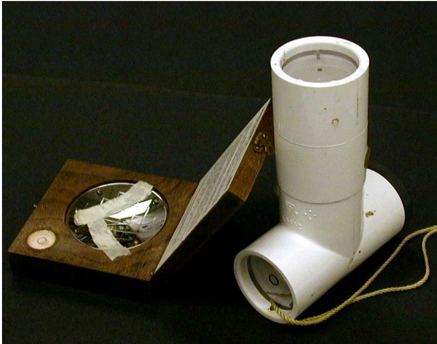
Figure 3. The concave spherical densiometer with tape for Strickler's modification is on the left and the vertical sighting tube is on the right.
